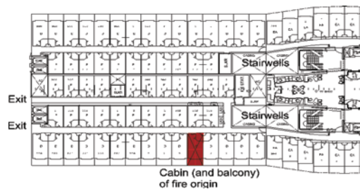
Figure 2. The cruise ship accommodation deck showing the cabin (with balcony) of fire origin, the exits and the stairwells.
